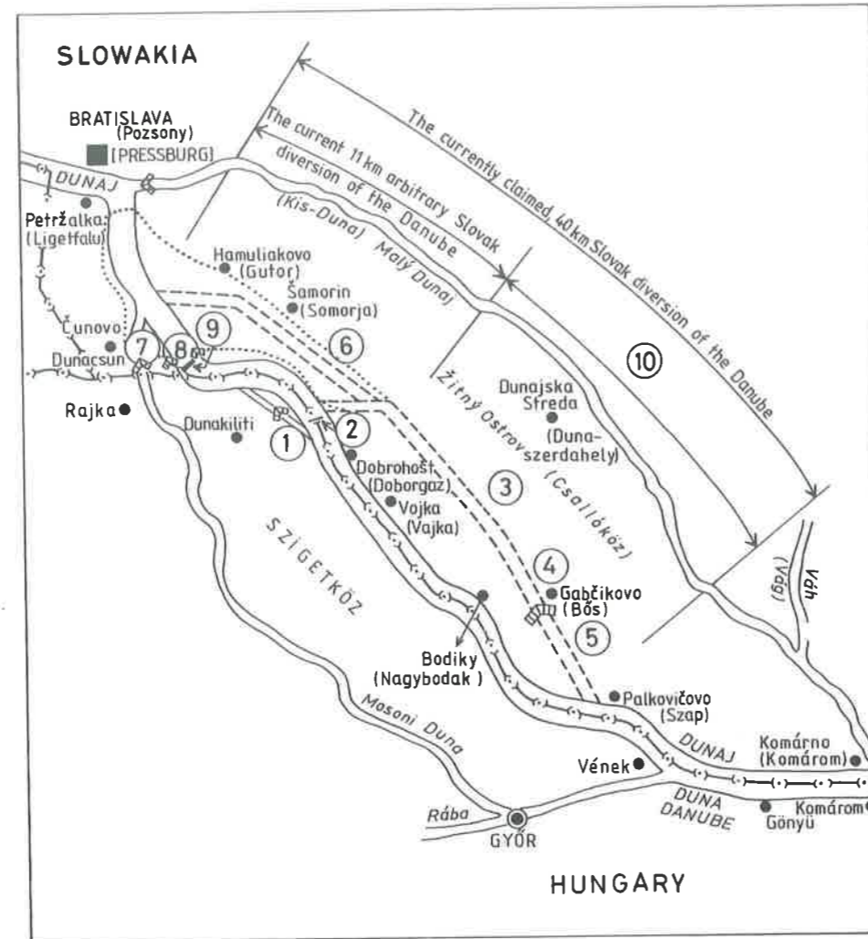
Fig. 37. General layout of the diversion of the Danube, the Variant C. Explanation: 1 = the Dunakiliti dam completed but not in operation; 2 = the planned but stopped Dunakiliti river-bed closure; 3 = the Gabčíkovo upstream canal; 4 = the Gabčíkovo barrage; 5 = the Gabčíkovo downstream canal; 6 = the arbitrary extended Gabčíkovo upstream canal, built illegally; 7 = the new flood-gate of the Mosoni-Duna; 8 = the Čunovo dam, built not in accordance with the agreement; 9 = the arbitrary planned Čunovo river-bed closure; 10 = the proposed 29 km diversion of the Danube in accordance with the 1977 agreement
